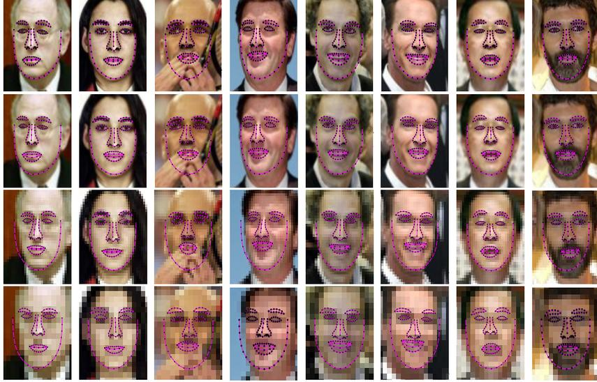
Figure 2.5: Example face shape detections for the LFW database using KRR with pixel features. Starting from the top row we display results for  $250 \times 250$  pixel face images which have been normalized to a 42, 20, 10, and 5 pixel inter-eye distance.
